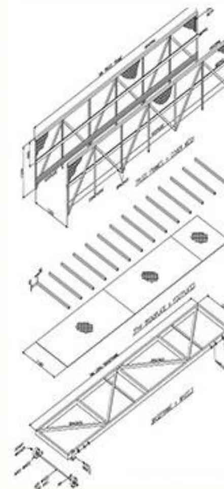
The hand railing used on our gangways also complies with BS MA 78:1978 but where the gangway is used at a severe incline, the height of the handrail is increased and non-slip slats are laid across the flooring to give
